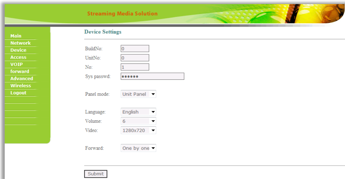
Figure 25: Device Settings Interface of the Outdoor Intercom
