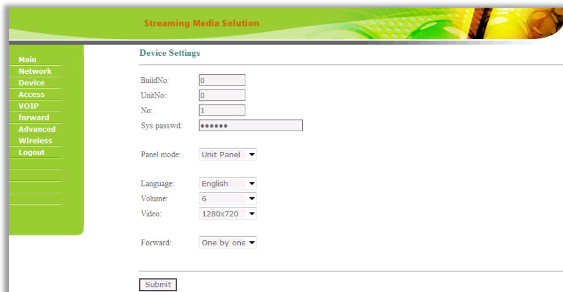
Figure 25: Device Settings Interface of the Outdoor Intercom
