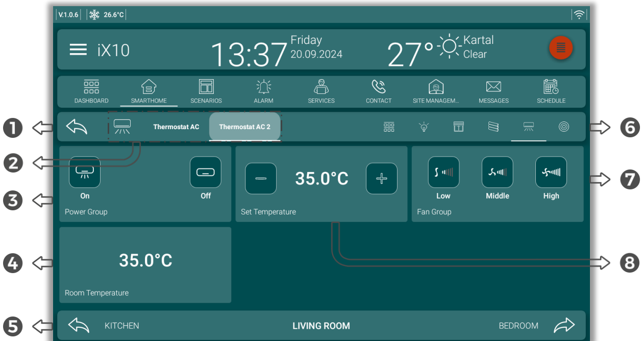
Fig. 14: Air Conditioner Section
