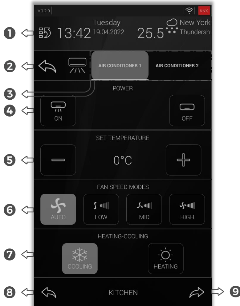
Fig. 13: Air Conditioner Section
