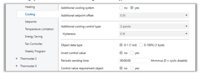
Fig. 54: Additional Cooling System Configuration Page
