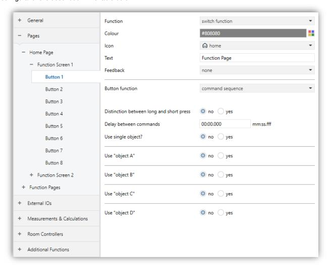
Fig. 18: Command Sequence Function Configuration Page
