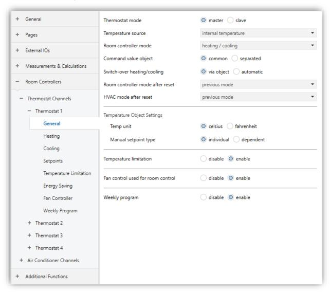
Fig. 44: Room Controller Thermostat General Configuration Page
