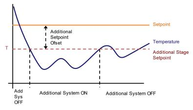
Fig. 50: PI Continuous Graph for Additional Heating Control
