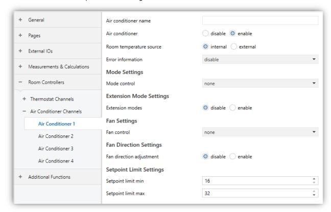
Fig. 67: Air Conditioner X Configuration
