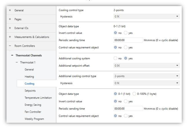
Fig. 51: Cooling 2-Points Control Configuration Page
