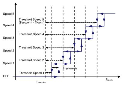
Fig. 63: Fan Controller 2-Points Control Cycle for Cooling
