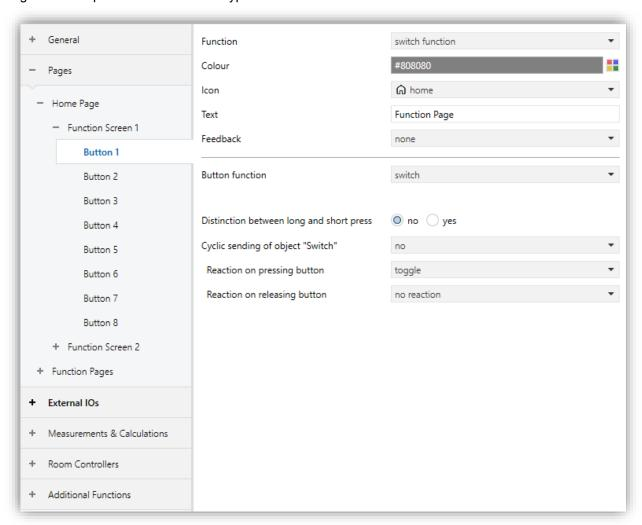
Fig. 12: Switching Function Configuration Page
