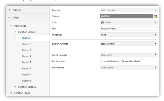
Fig. 16: Scene Control Function Configuration Page
