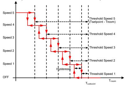
Fig. 62: Fan Controller 2-Points Control Cycle for Heating
