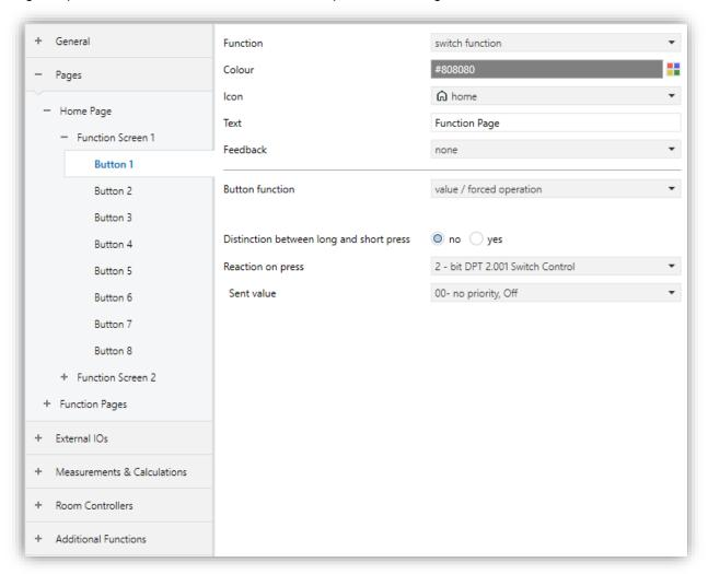
Fig. 15: Value/Forced Operation Function Configuration Page
