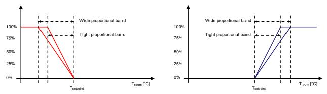
Fig. 65: Fan Controller Proportional Control
