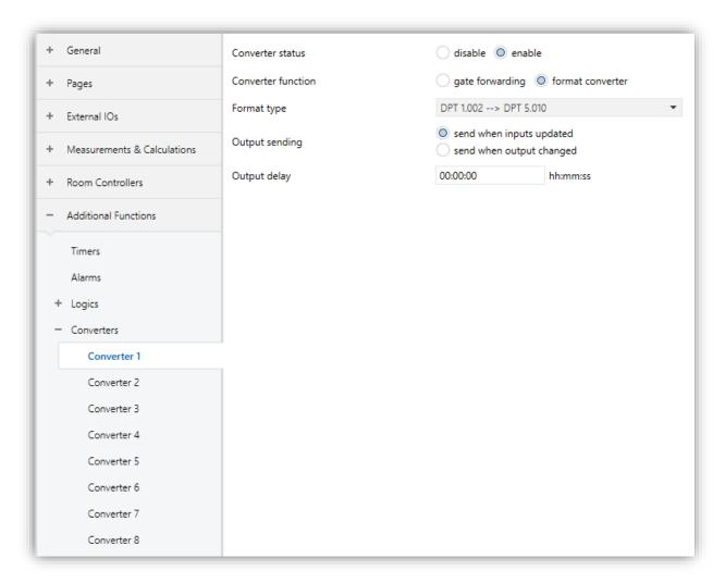
Fig. 82: Logics - Format Converter Configuration Page
