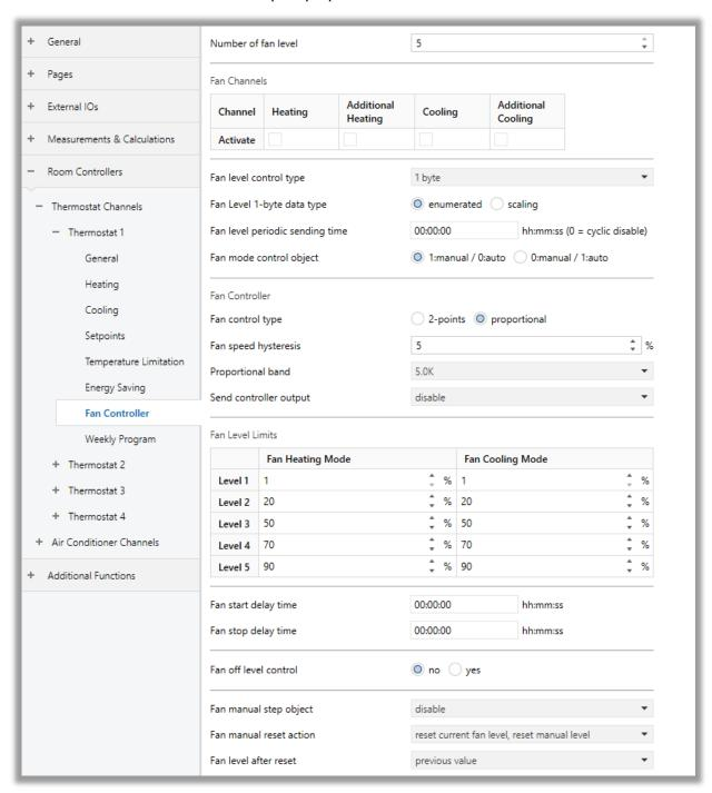
Fig. 64: Fan Controller Proportional Control Configuration
