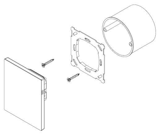
Fig. 3: Mounting the to Flush Mounting Box
