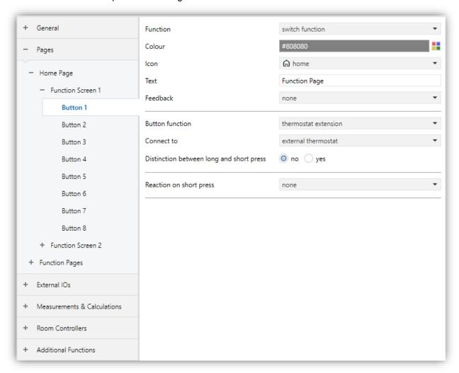
Fig. 22: Thermostat Extension Configuration Page
