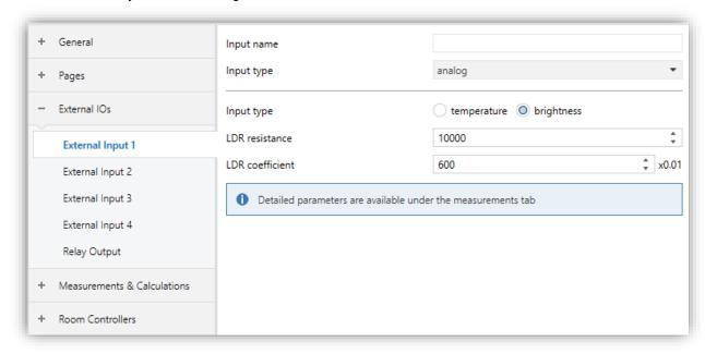
Fig. 27: Analog Input - Brightness Page
