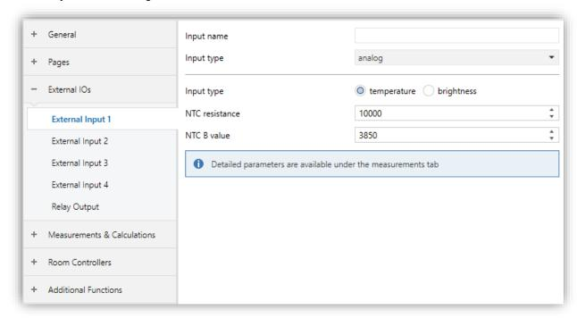
Fig. 26: Analog Input – Temperature Page
