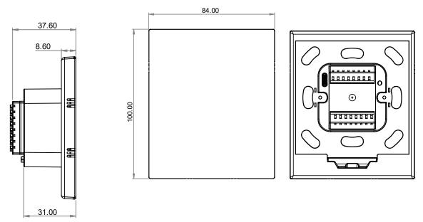
Fig. 1: Dimensions of the iX4
