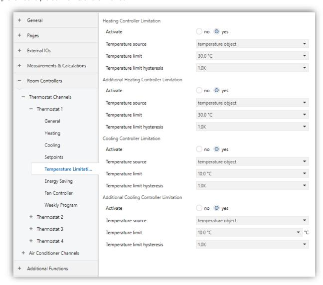
Fig. 59: Temperature Limitation Configuration Page
