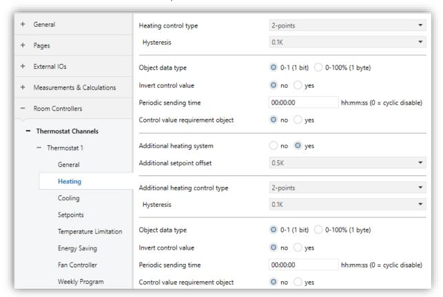
Fig. 45: Heating 2-Points Control Configuration Page
