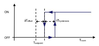
Fig. 55: 2 – Points Hysteresis Cycle for Additional Cooling Control
