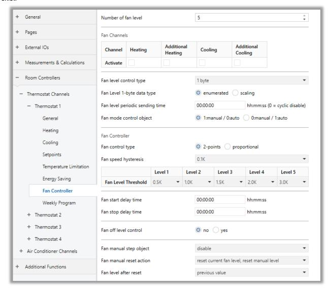
Fig. 61: Fan Controller 2-Points Control Configuration Page
