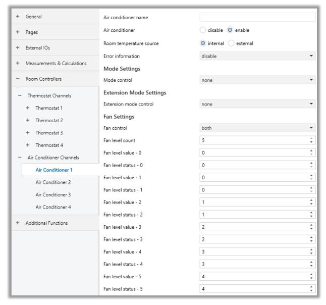
Fig. 70: Air Conditioner – Fan Settings Configuration Page
