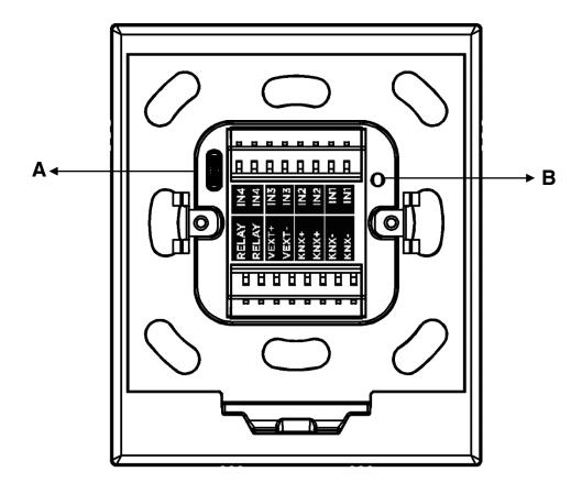
Fig. 2: Connection to KNX and Programming Button
