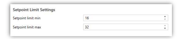
Fig. 72: Air Conditioner – Setpoint Limit Settings Configuration Page
