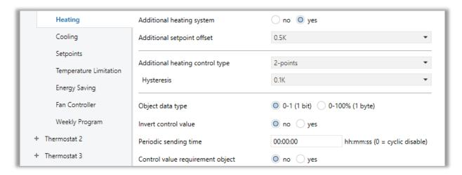
Fig. 48: Additional Heating System Configuration Page
