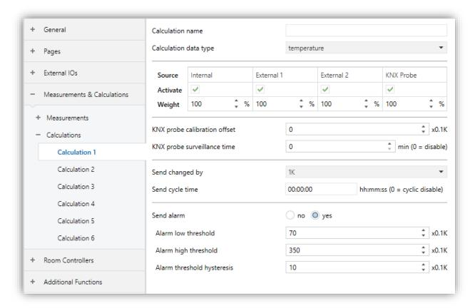
Fig. 39: Calculation for Temperature Page
