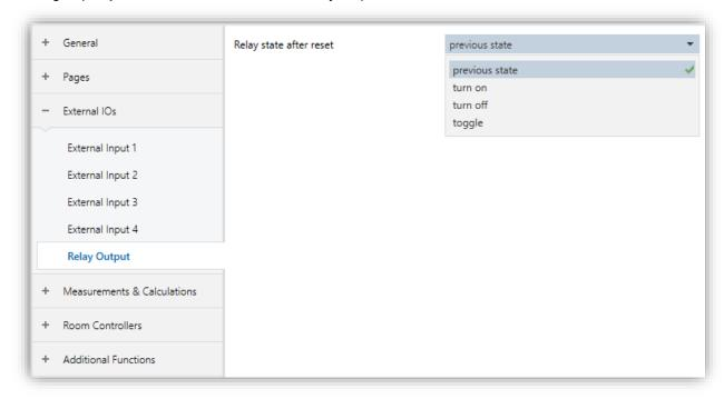
Fig. 30: Relay Output Configuration Page
