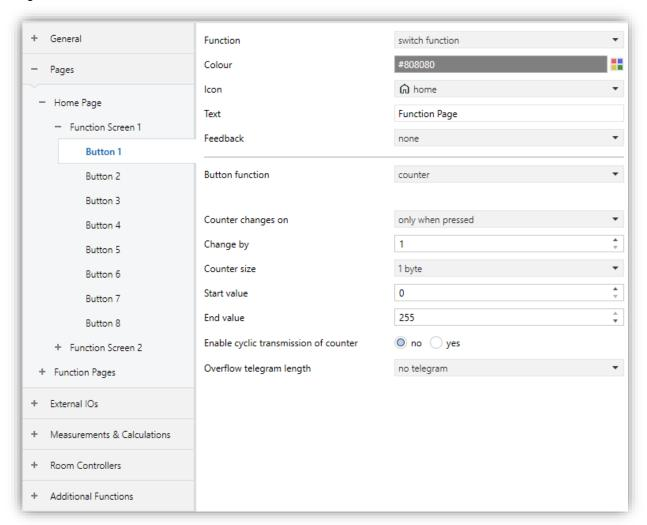
Fig. 19: Counter Function Configuration Page
