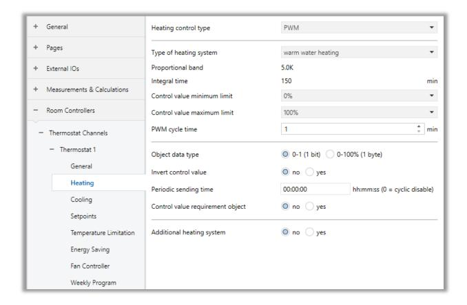
Fig. 46: Heating PWM Control Configuration Page
