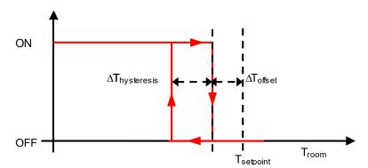
Fig. 49: 2 – Points Hysteresis Cycle for Additional Heating Control
