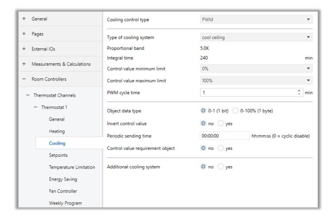
Fig. 52: Cooling PWM Control Configuration Page
