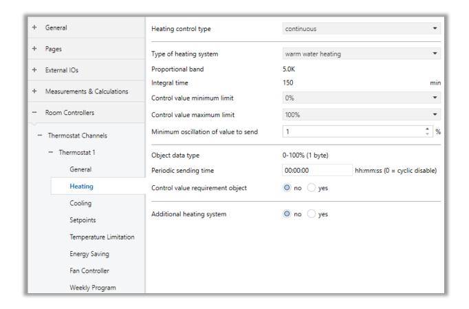
Fig. 47: Heating Continuous Control Configuration Page
