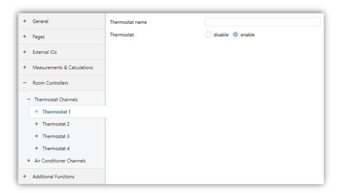
Fig. 43: Room Controller Thermostat Configuration Page
