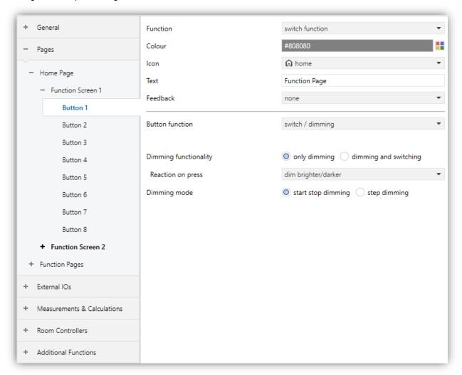
Fig. 13: Switch/Dimming Function Configuration Page
