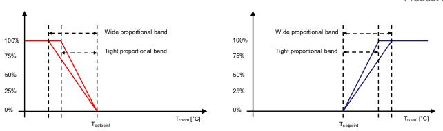
Fig. 41: Continuous PI Control Proportional Band Widths
