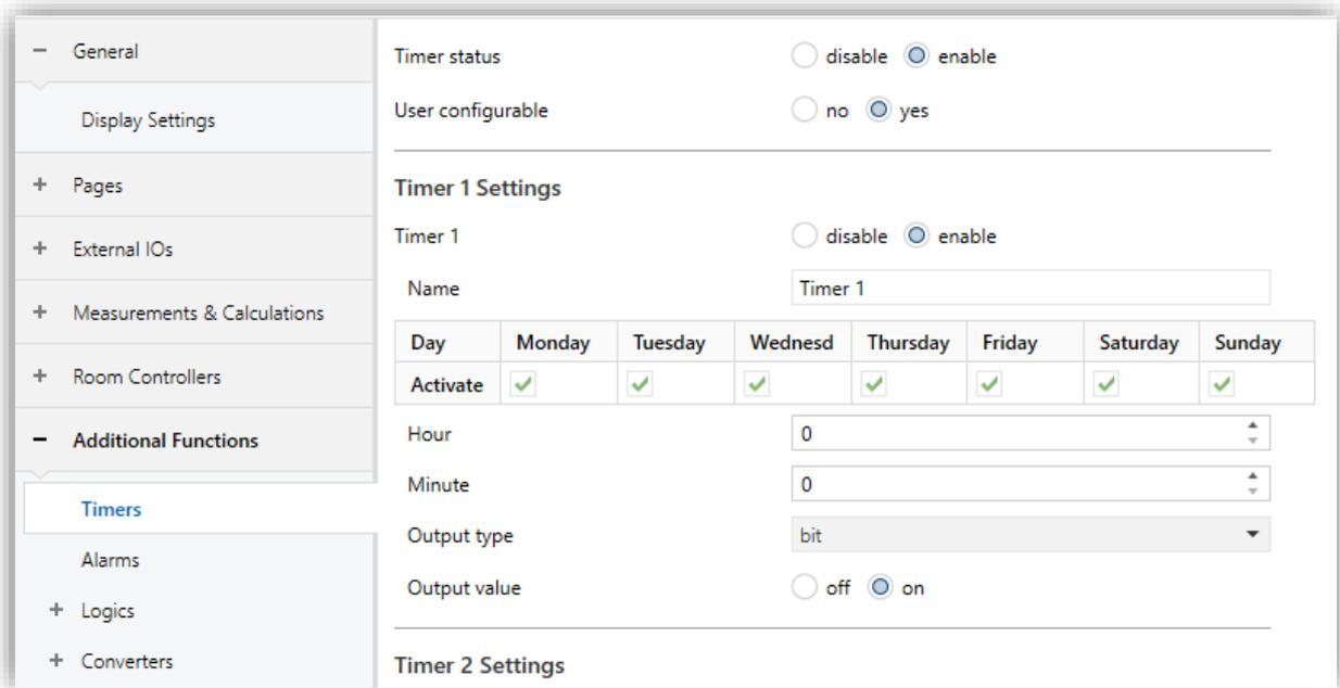
Fig. 73: Additional Functions – Timers Configuration Page
