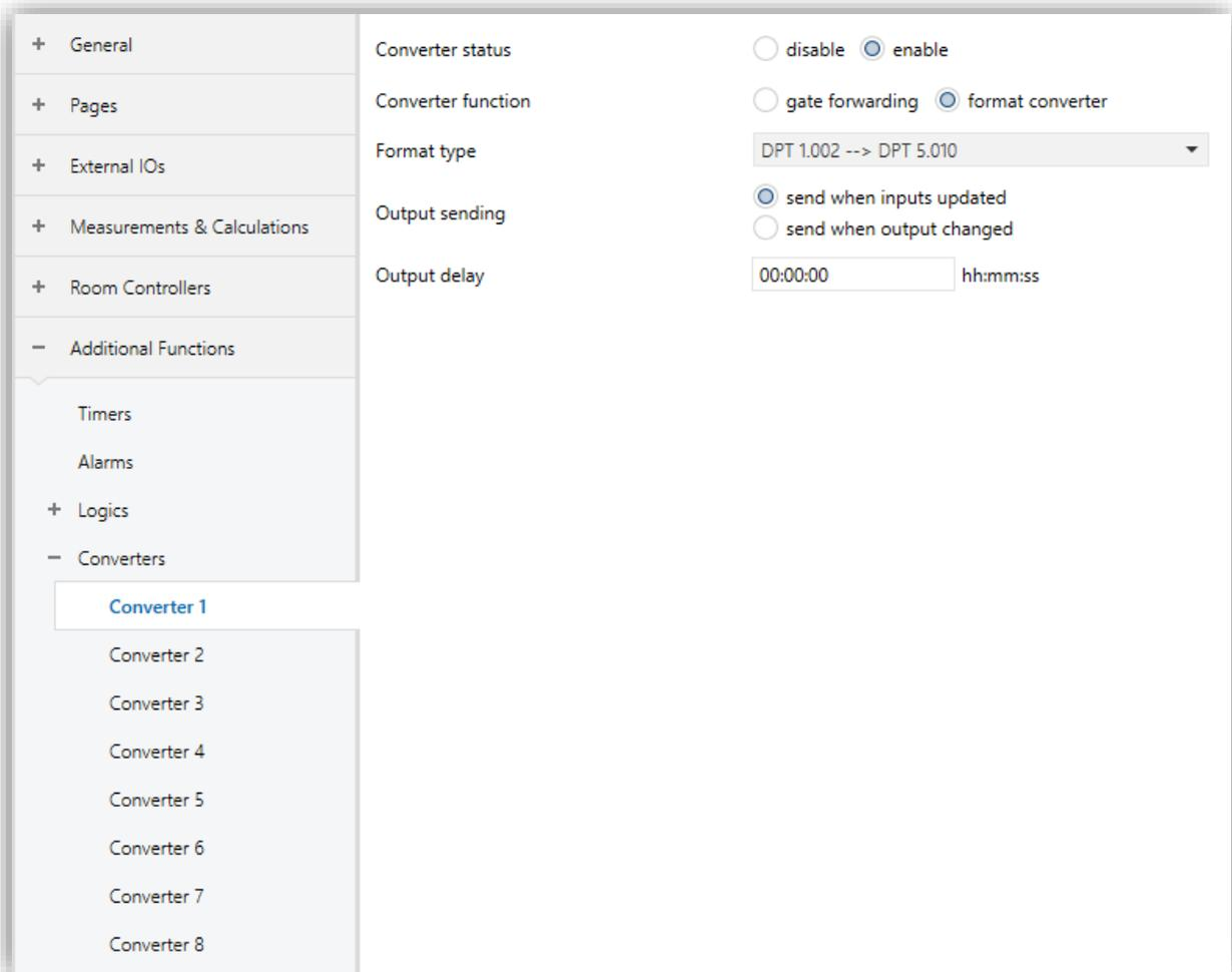
Fig. 82: Logics – Format Converter Configuration Page
