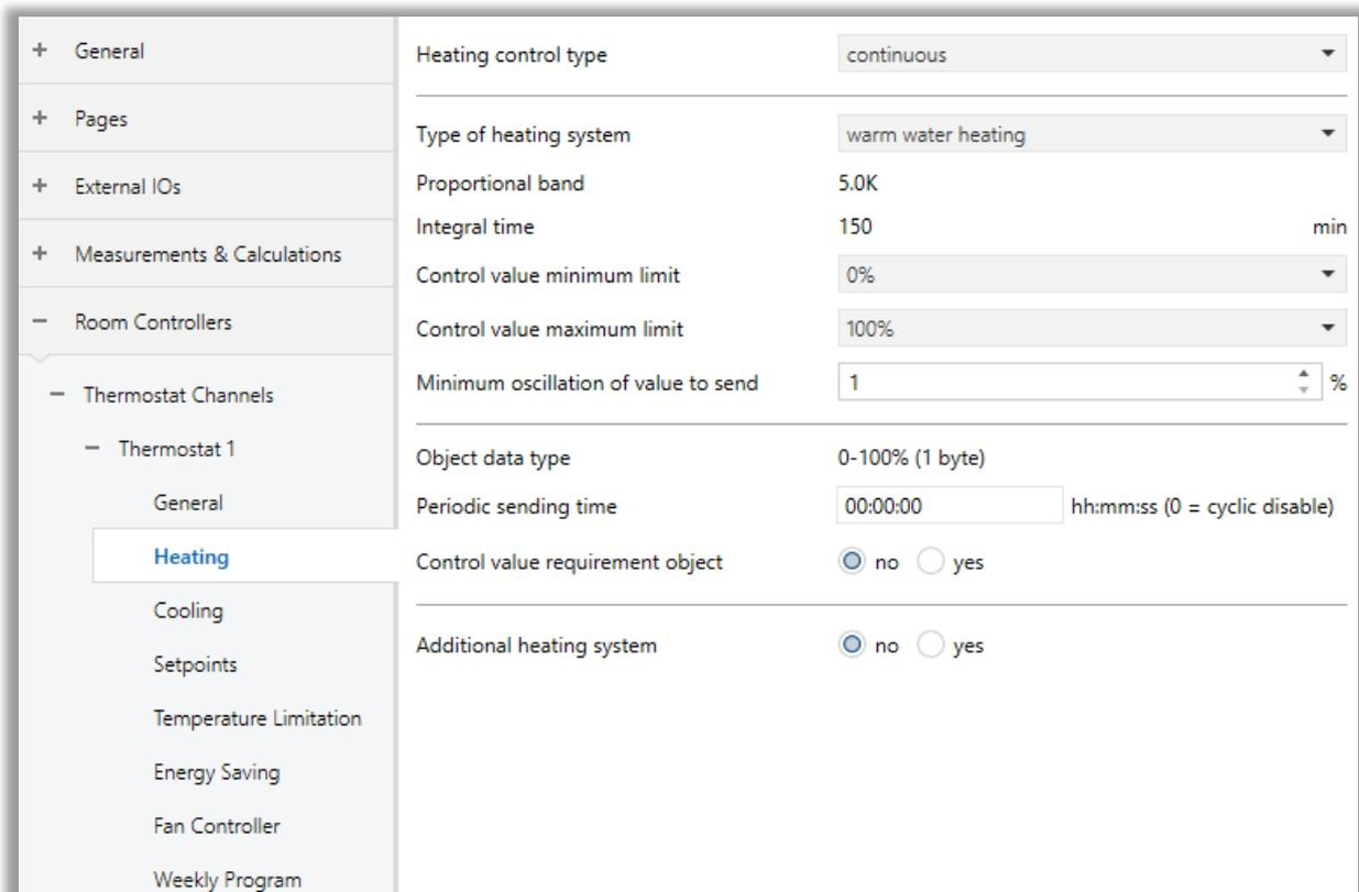
Fig. 47: Heating Continuous Control Configuration Page
