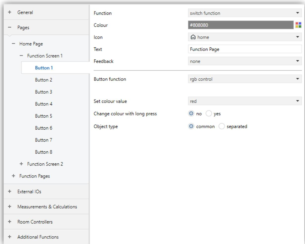
**Fig. 20:** RGB Colour Control Function Configuration Page
