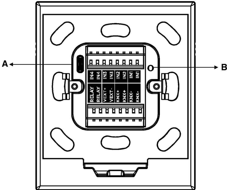
**Fig. 2:** Connection to KNX and Programming Button
