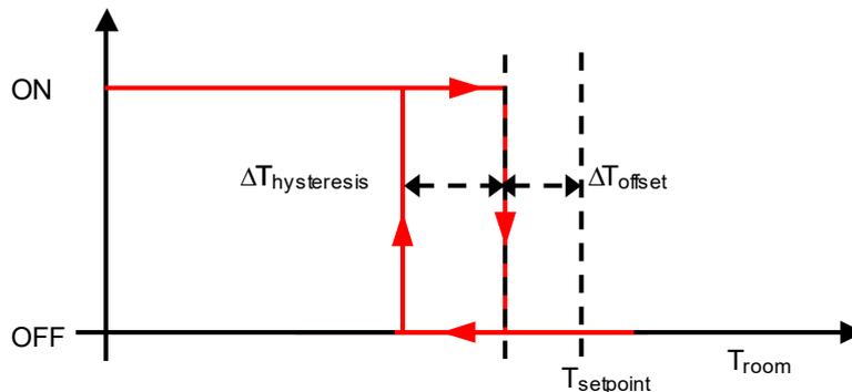
Fig. 49: 2 – Points Hysteresis Cycle for Additional Heating Control
