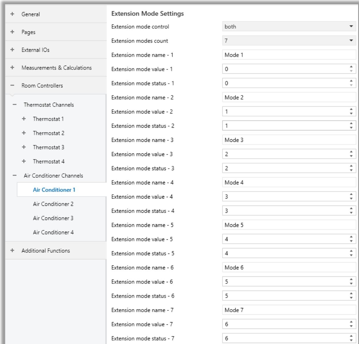
Fig. 69: Air Conditioner – Extension Mode Settings Configuration Pages
