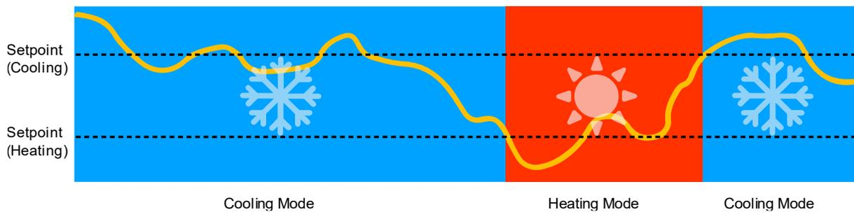
**Fig. 57:** Automatic Heating & Cooling Mode Switch
