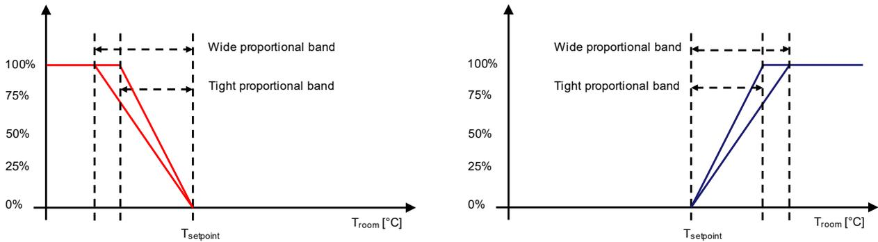
Fig. 41: Continuous PI Control Proportional Band Widths
