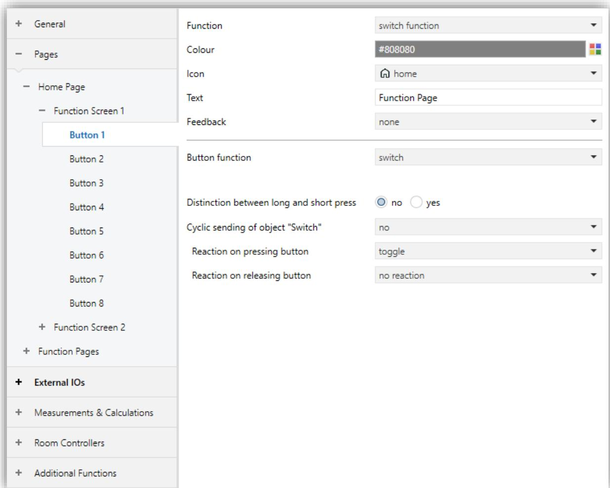
Fig. 12: Switching Function Configuration Page
