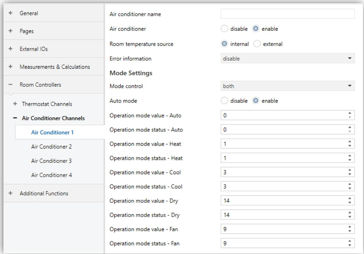
Fig. 68: Air Conditioner X – Mode Settings Configuration Page
