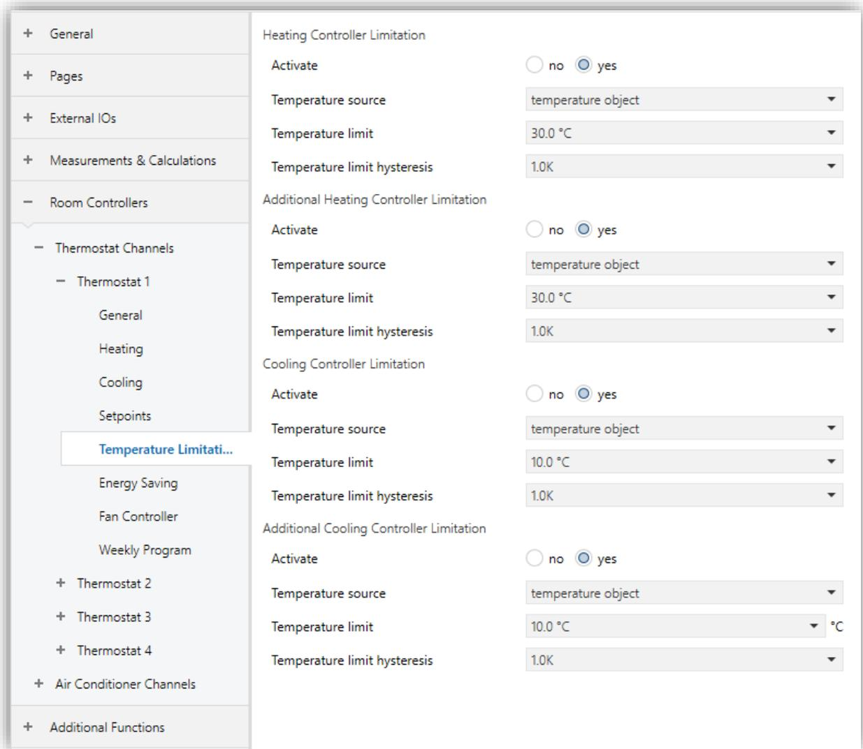
Fig. 59: Temperature Limitation Configuration Page
