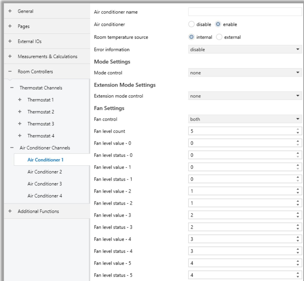
Fig. 70: Air Conditioner – Fan Settings Configuration Page
