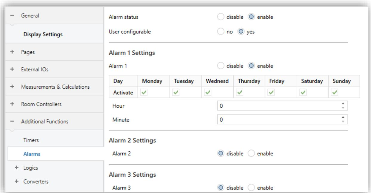
Fig. 74: Additional Functions – Alarms Configuration Page
