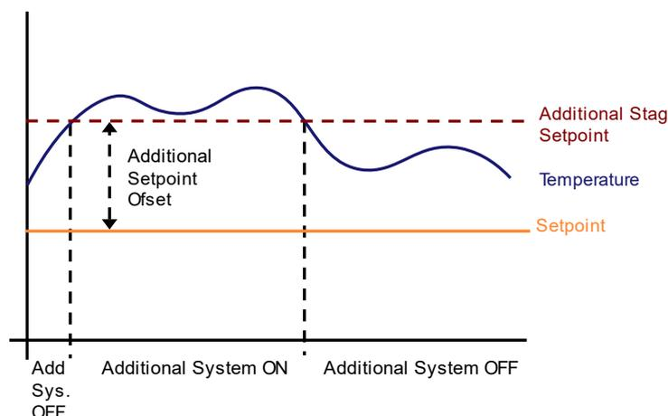
Fig. 56: PI Continuous Graph for Additional Cooling Control
