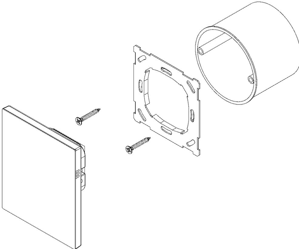
**Fig. 3:** Mounting the to Flush Mounting Box
