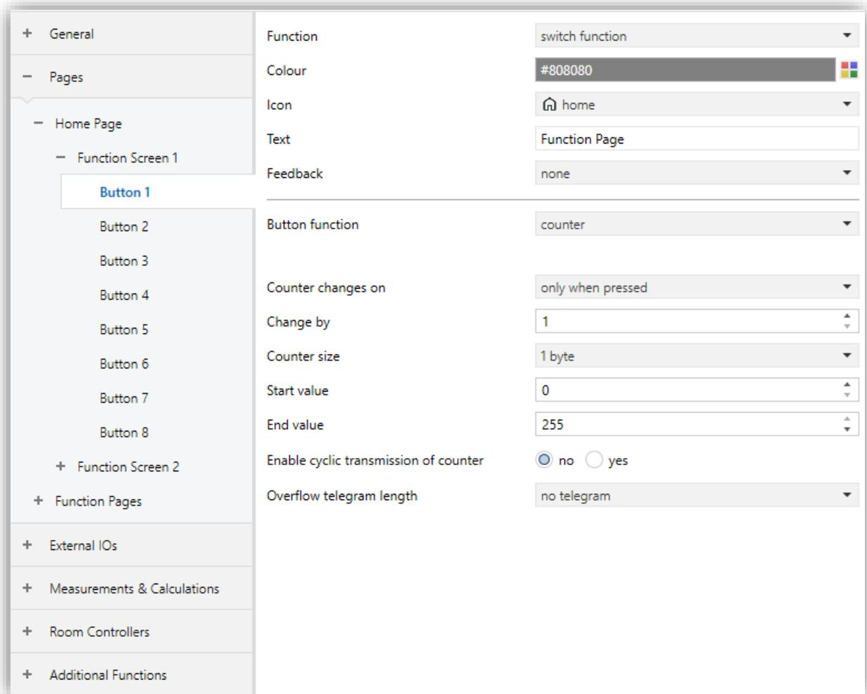
Fig. 19: Counter Function Configuration Page
