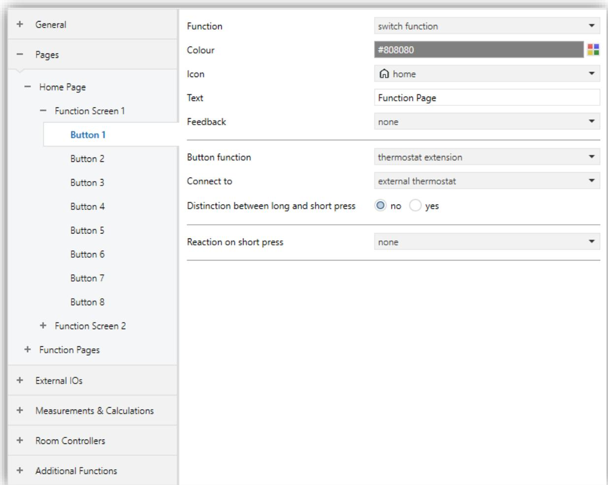
**Fig. 22:** Thermostat Extension Configuration Page
