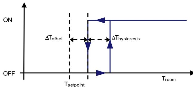
Fig. 55: 2 – Points Hysteresis Cycle for Additional Cooling Control
