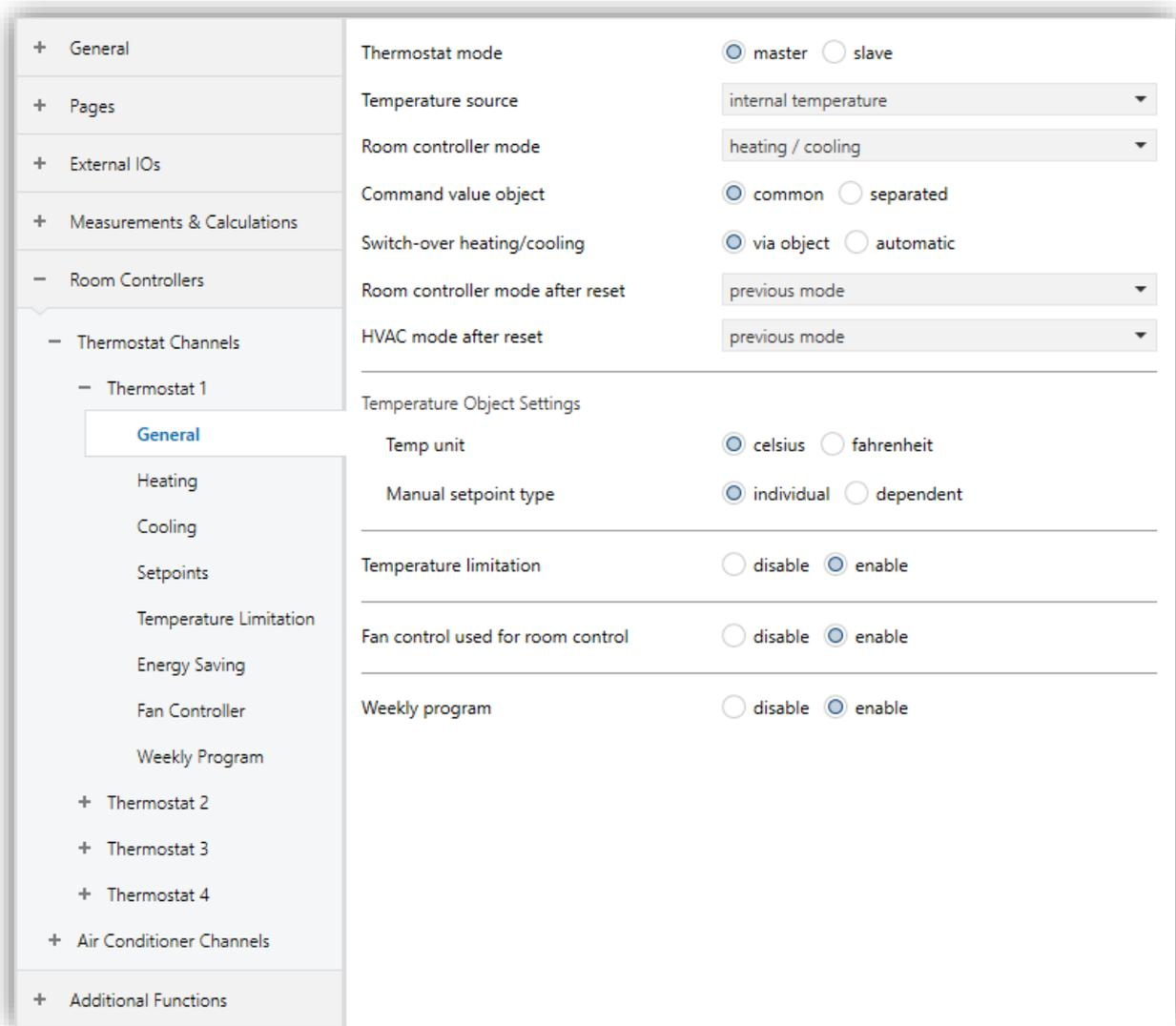
Fig. 44: Room Controller Thermostat General Configuration Page
