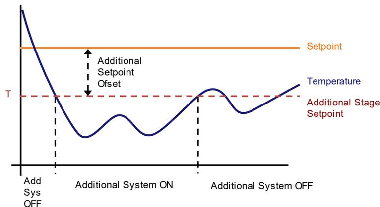
Fig. 50: PI Continuous Graph for Additional Heating Control
