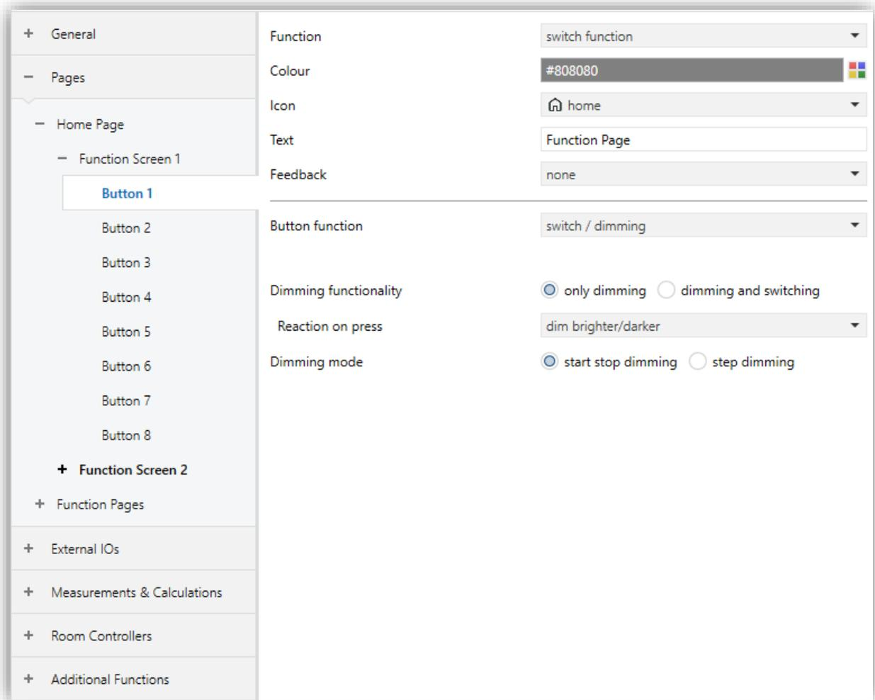
Fig. 13: Switch/Dimming Function Configuration Page
