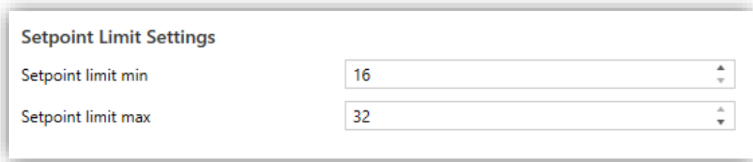
Fig. 72: Air Conditioner – Setpoint Limit Settings Configuration Page
