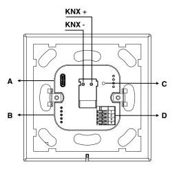
A USB Port B Upgrade Port C KNX Programming Button **D** Inputs
