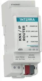
ITR902-0001 - KNX / IP Router is a KNXnet/IP routing and tunneling device that connects the KNX line and Ethernet network. The device can also be used as a KNX IP line coupler without requiring any power supply.
