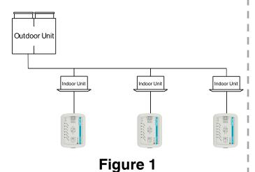
Carrier VRF AC - KNX Gateway can be connected directly to the wired remote communication bus terminal of the AC indoor unit.
