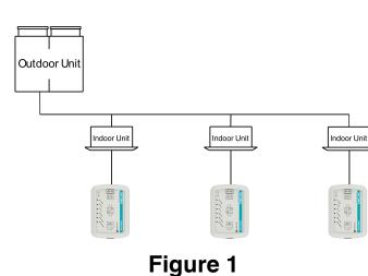
Alarko VRF AC - KNX Gateway can be connected directly to the wired remote communication bus terminal of the AC indoor unit.
