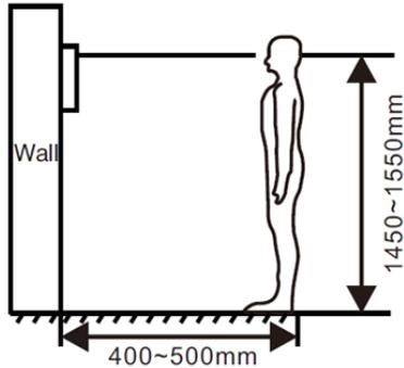
**!** During the installation, the camera should be 1450-1550 mm above the ground. The camera tether for photographing the human face should be the top priority.
