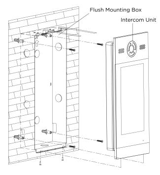
The following figure, shows the proper location of the installation:
