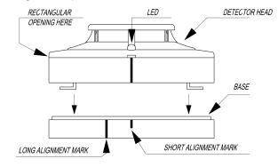
2. Mate the detector head onto the base and twist clockwise to secure it.
