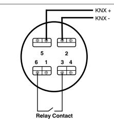
**INTERRA KNX SMOKE + HEAT DETECTOR LAYOUT**
