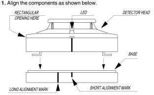
2. Mate the detector head onto the base and twist clockwise to secure
