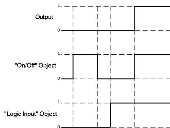
Fig8. AND Logic Function
