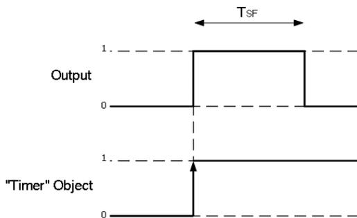
Fig2. Staircase Function
