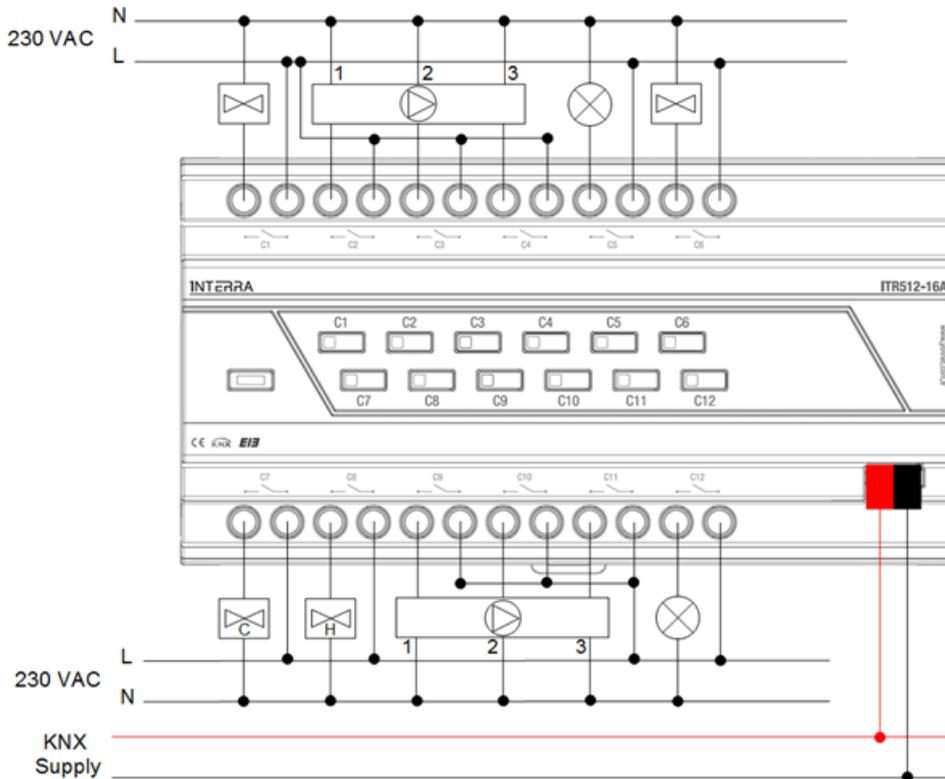
Fig22. Connection Diagram Example Configuration 2
