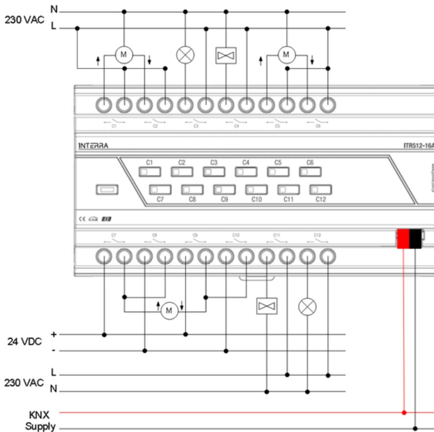
Fig23. Connection Diagram Example Configuration 3
