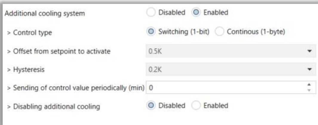
Fig. 38: Additional Cooling System Configuration
