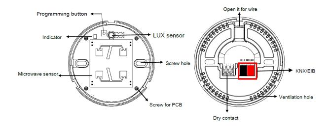
Fig 2: KNX Connector, Programming LED and Button.
