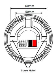
Fig 4: Screw Holes Used in Mounting the Device
