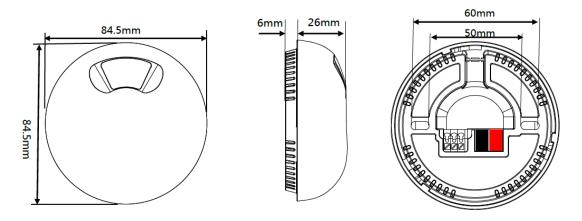
Fig 1: Front, Side and Rear Appearances and Measures of the Device.
