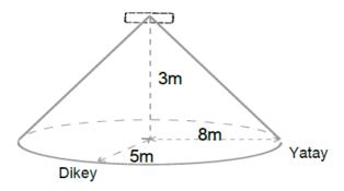
Fig 3: Microwave Sensor Detection Diagram.
