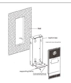
When mounting the built-in box, do not fix the frame into the wall. The supporting frame should be in parallel with the wall.
