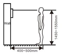
During the installation, the camera should be 1450-1550 mm above the ground. The camera tether for photographing the human face should be the top priority.
